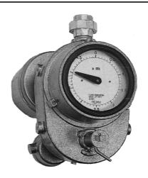
The rotation angle of the sprocket pulley shaft is transmitted to the pointer through the gear mechanism, and the liquid level is indicated by the pointer and the scale plate, or by the counter.
